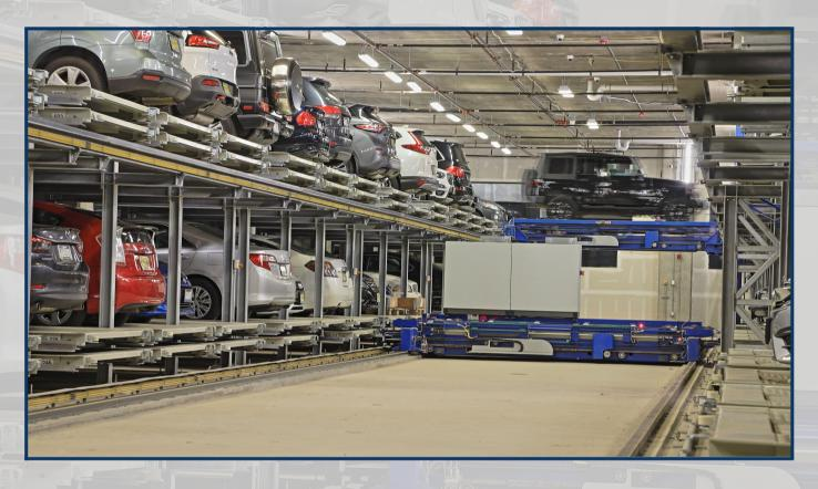
Based on a modular concept, the SP can be adapted to meet the specific requirements of any given location. Through the combination of vertical car elevators passing through the entire system and shuttles that work on each individual parking level, the SP boasts a limitless array of possible configurations. The SP provides several hundred parking spots that can be built above or below grade.
