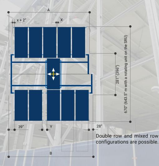
Parking spots on concrete ceilings require the pallet distance X = 4.75" without wall plates and Y = thickness of the wall plate + 11".
