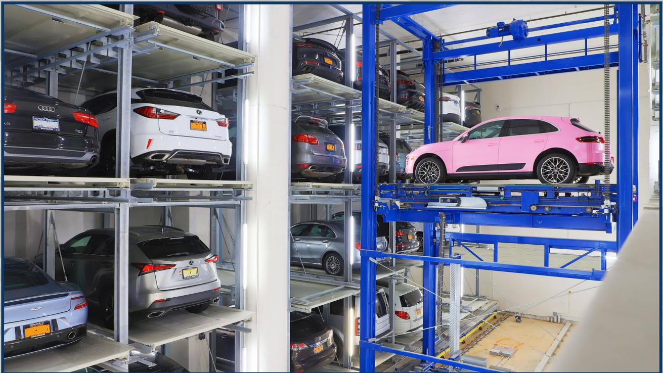
Our UP System is the Universal parking system that gives you the option to build more parking spaces economically in office buildings or as a public parking system. With AutoMotion's UP System, up to 100 parking places for various vehicles can be accommodated using only 1 Storage and Retrieval Unit (SRU) at a maximum height of 65.7 ft. With AutoMotion UP System, our parking solution's rack structure can be built above-ground, below-ground, or in a mixed-solution type of parking.
